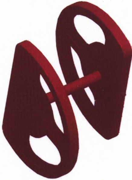
Figure 3.10 Driver Disk Interference Cut out Feature
