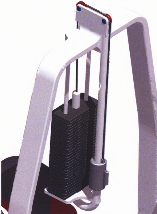
Figure 3.17 Weight Suspension System
