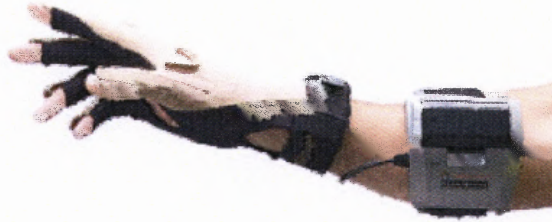
Figure 3.4 The CyberGlove® II System: Wireless Data Glove from Immersion. ( http://www.immersion.com/3d/products/cyber_glove.php )
