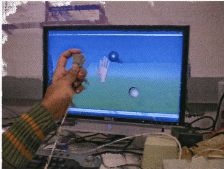
Figure 3.2 Simple game displaying hand motion tracked in VRML using FOB.
