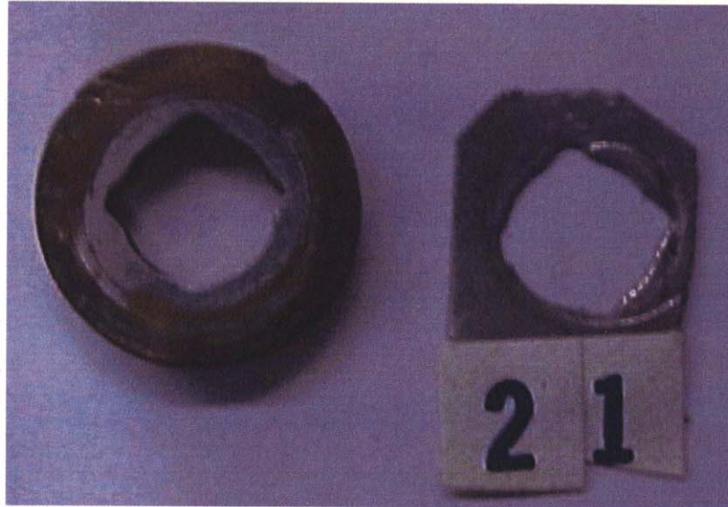
Figure 3.9 Piercing an irregular opening in a stainless steel plate. Opening diameter is ~3 times larger extruder nozzle diameter.
