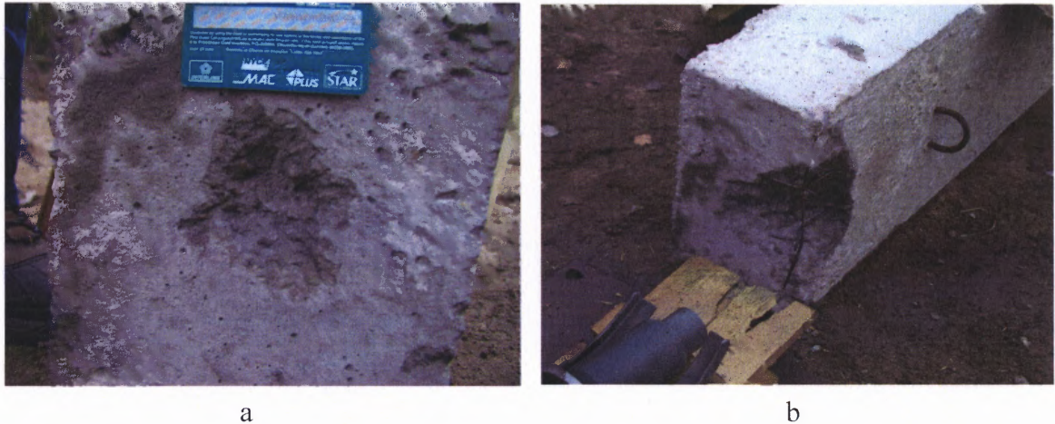
Figure 4.11 Results of two consequent shots to a butt of an armored concrete block with reduced powder charge (30g of powder, 230g of water).
