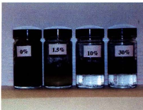
Figure 3.1 The four bottles contain 0, 1.5, 10, and 30% GAC/Aerogel composite respectively in a crude oil water mixture.
