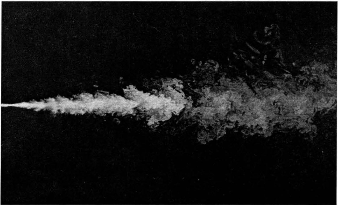
Figure 2.2 Example of a fully turbulent Jet (De Young, 2004).
