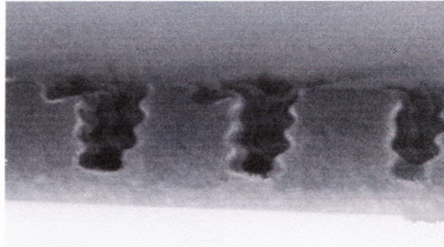
Figure 4.2 SEM image of vertical standing wave causing additional exposure.
