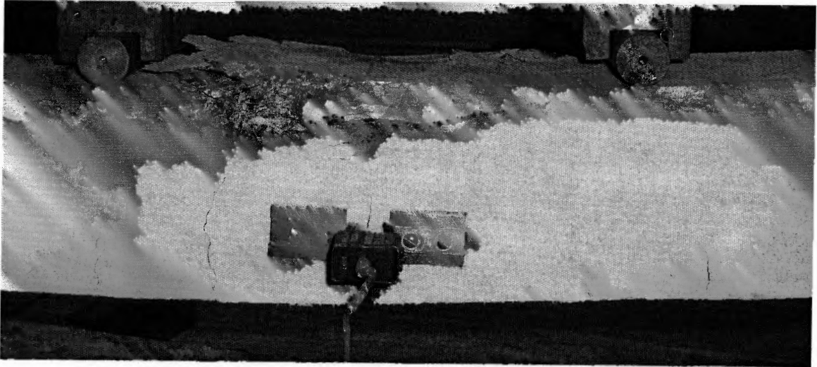
(a) Failure of Over-reinforced concrete
