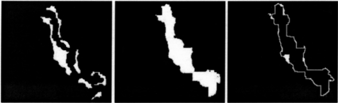
Figure 4.6 Left: result of component labeling; middle: result of the final model; right: result of differences between the current and previous images.
