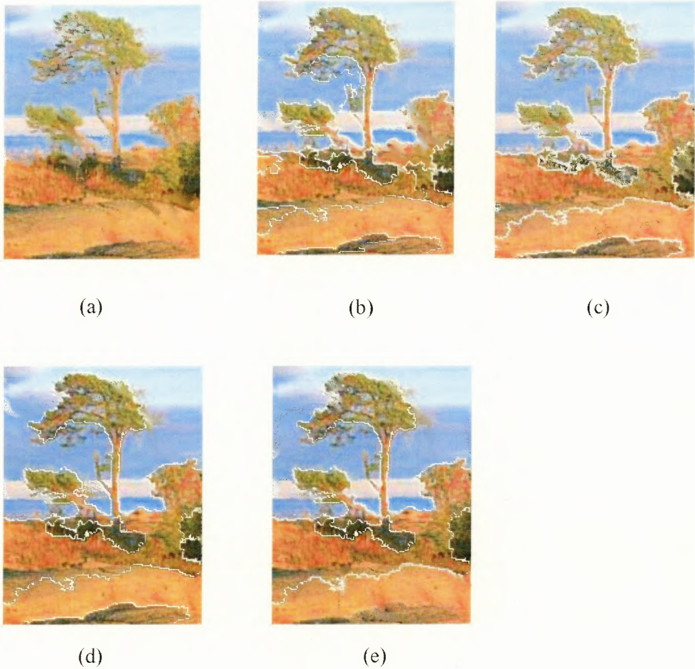
Figure 2.1.5 Example of choosing the relative Euclidean distance threshold for further region merging. (a) Original image, (b) the result after merging using 0.1 as the distance threshold value and 1/150 of the image size as the size threshold, (c) further merging using the relative Euclidean distance threshold 0.2, (d) further merging using threshold 0.15, and (e) further merging using threshold 0.25.
