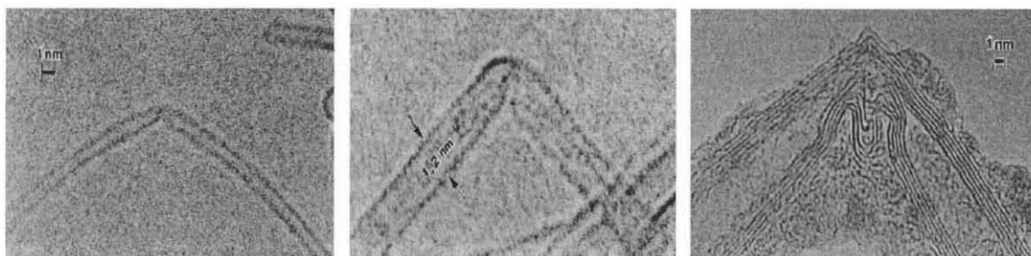
Figure 1.5 TEM images of SWNTs bent at different angles [17].
