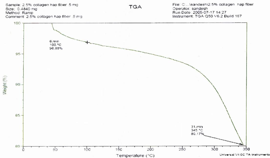
Figure A.4 Percentage Weight Retention in Collagen/Hydroxyapatite Composite Fiber.
