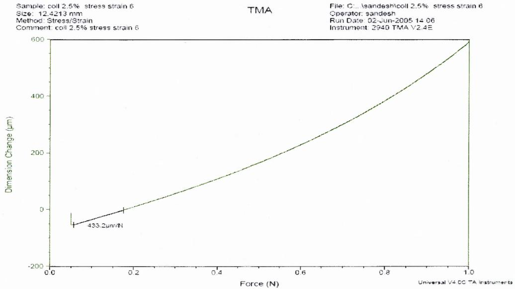
Figure C.1 Initial Tensile Modulus for Pure Collagen Fiber.
