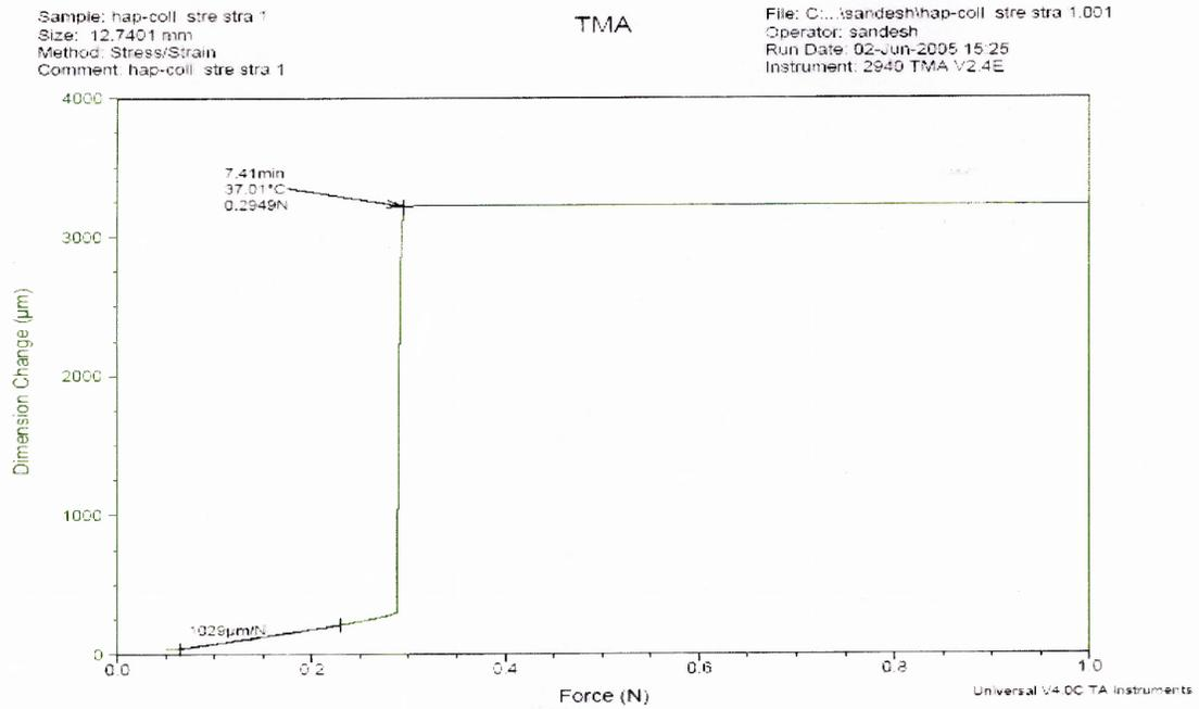
**Figure C.3** Initial Tensile Modulus for Collagen/Hydroxyapatite Composite Fiber.
