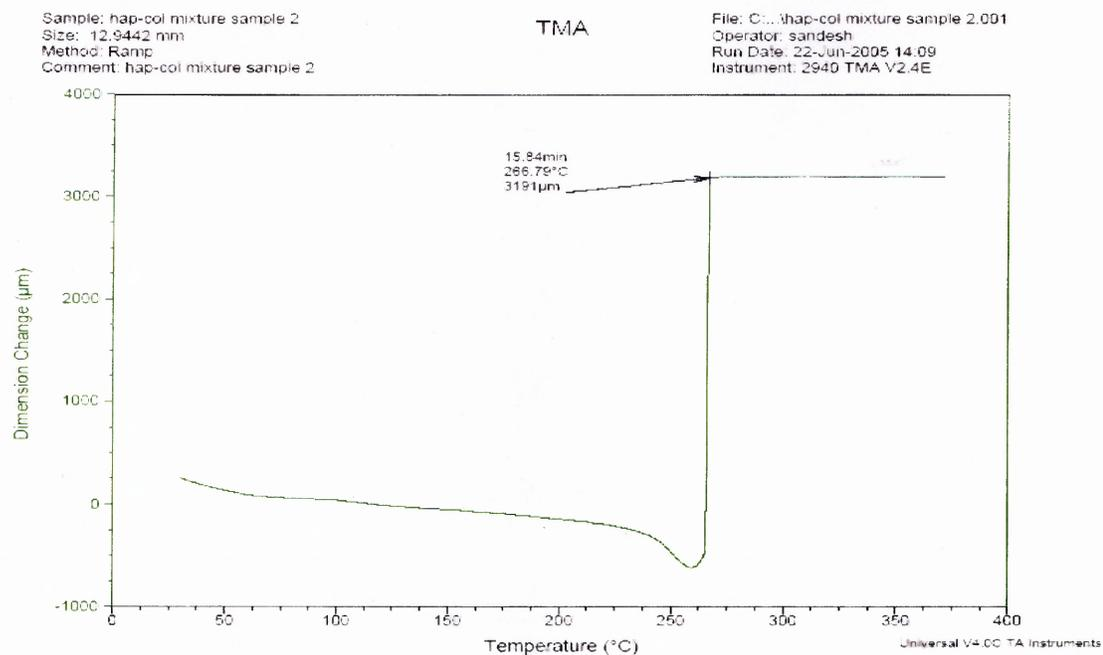
**Figure B.3** Breaking Point Temperature for Collagen/Hydroxyapatite Composite Fiber.
