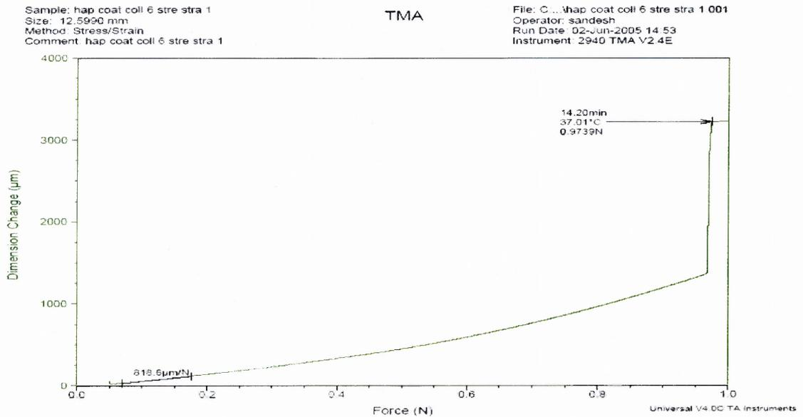
Figure C.2 Initial Tensile Modulus for HA coated Collagen Fiber.
