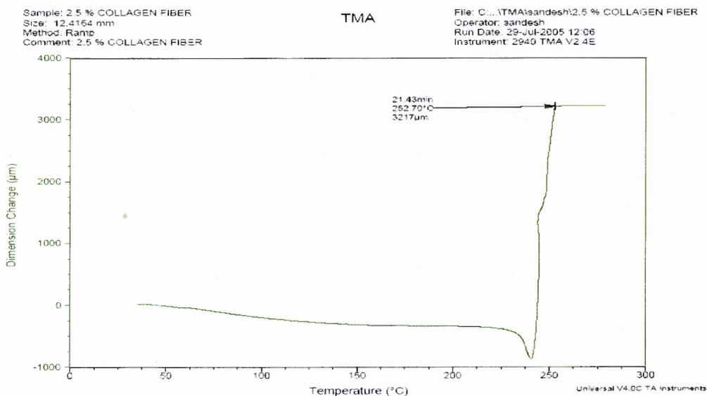
Figure B.1 Breaking Point Temperature for Pure Collagen Fiber.
