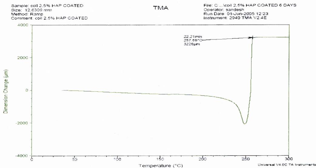
Figure B.2 Breaking Point Temperature for HA Coated Collagen Fiber.
