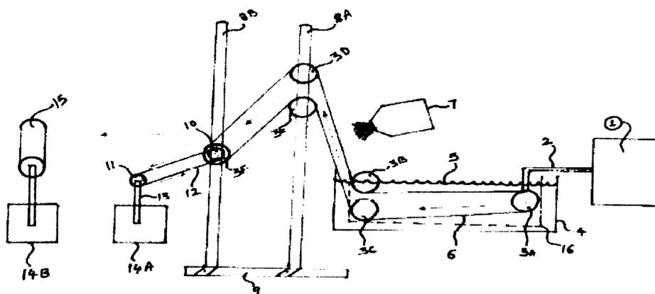
**Figure 3.1** Schematic Diagram of Wet Spinning Apparatus installed at MDCL.
