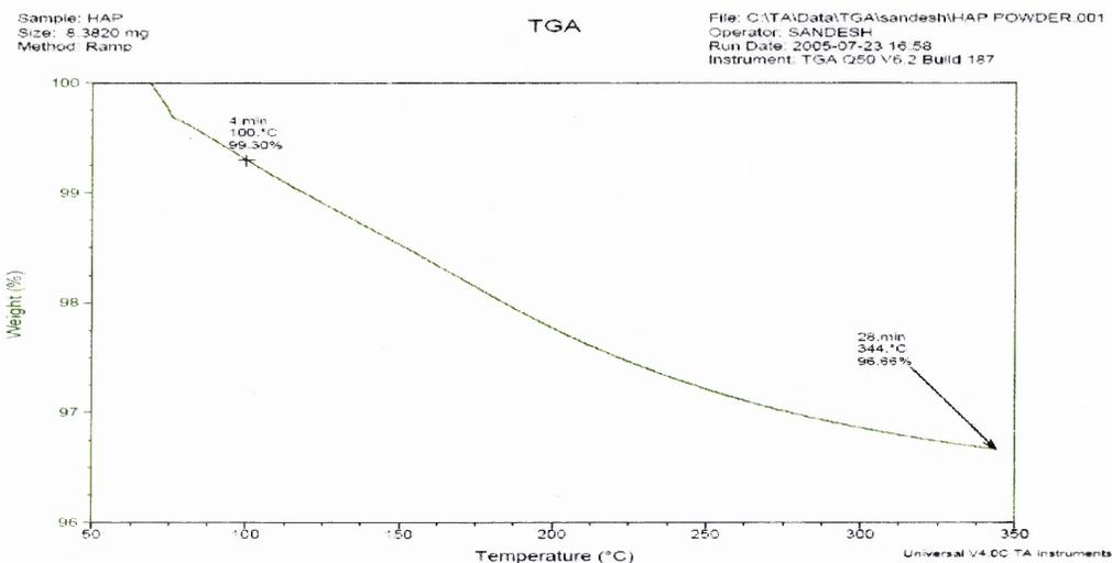
Figure A.1 Percentage Weight Retention for Hydroxyapatite Powder.
