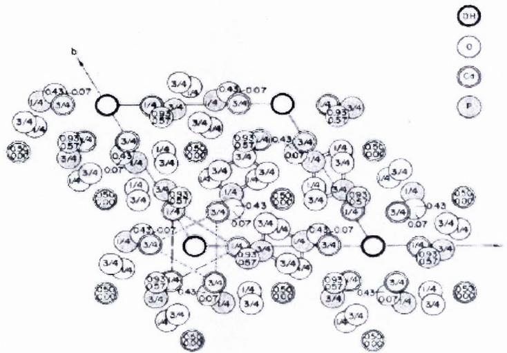
**Figure 2.5** Hydroxyapatite Structure Projected down C Axis onto Basal Plane [7].
