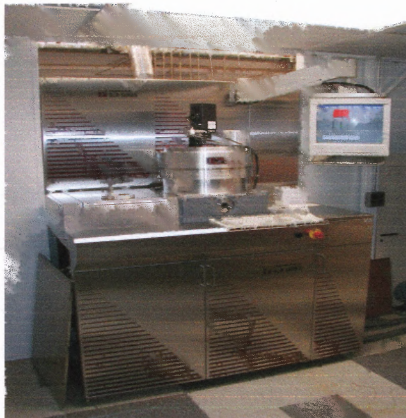
Figure 4.16 The deep reactive ion etching machine used in this study.
