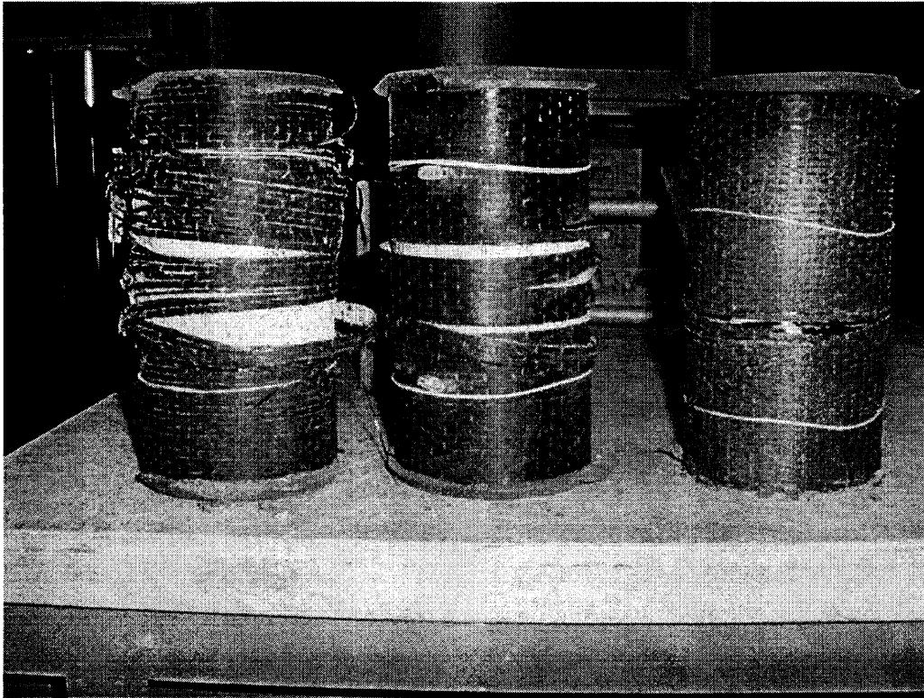
Figure 2.4 Failure conditions of CFRP strengthened specimens. (From left to right: 1 layer, 2 layers and 3 layers)
