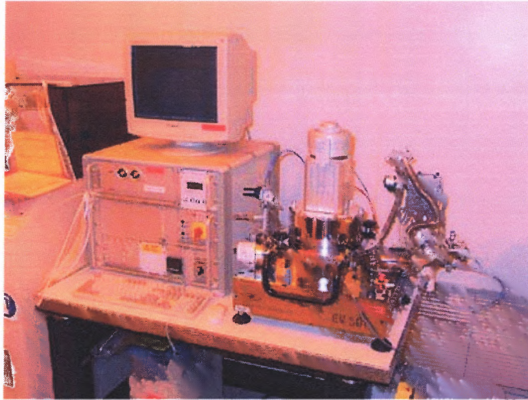
Figure 6.4 Photo of EV501 bonding station.
