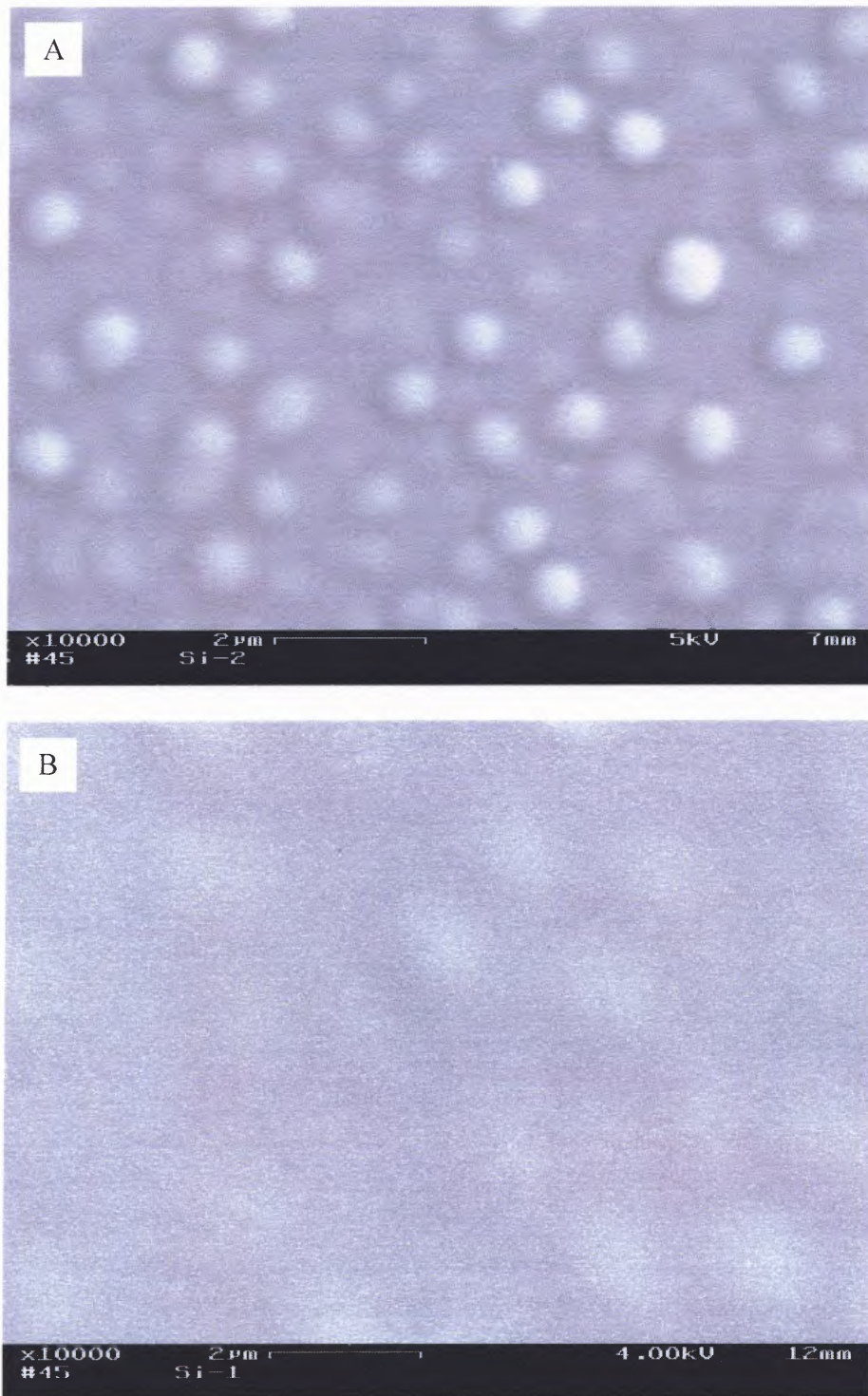
Figure 5.19 SEM pictures of silicon wafer's surface by H PIII (A) Center area, (B) Edge area.
