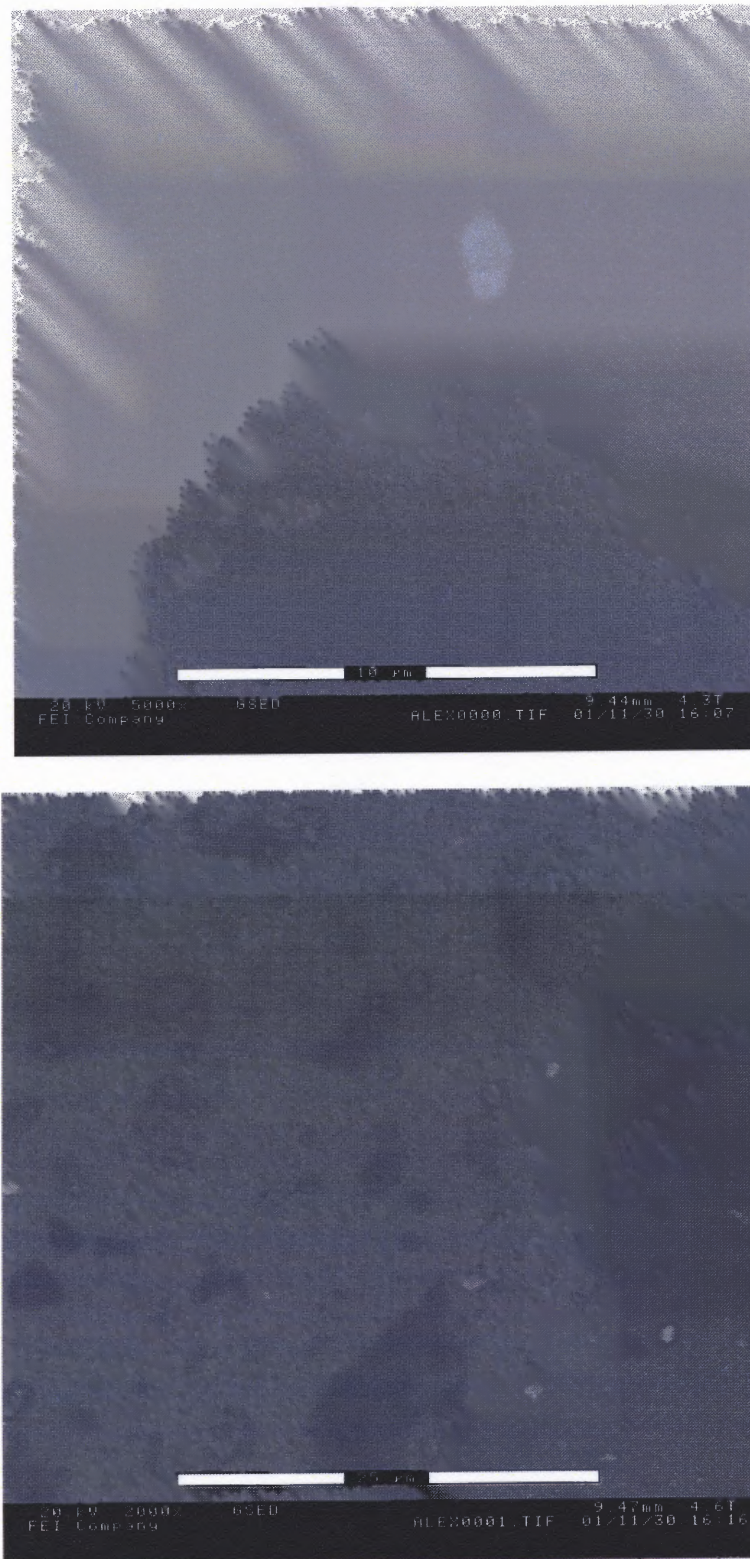
Figure 5.7 SEM pictures of Si samples surface after hydrogenation.
