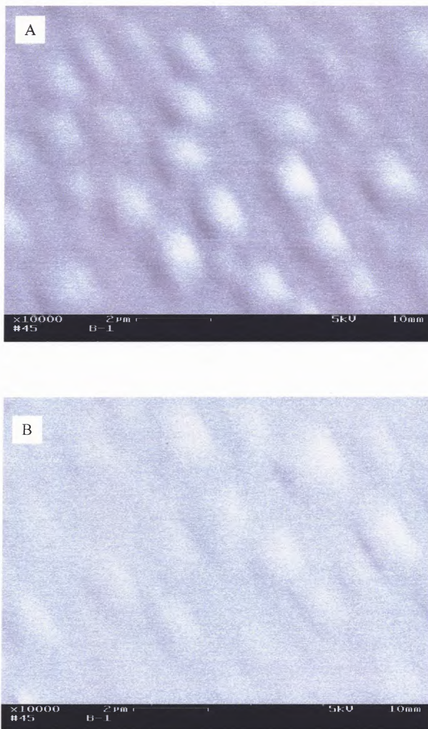
Figure 5.17 SEM pictures of silicon wafer's surface oby B implanted, then H PIII (A) Center area, (B) Edge area.
