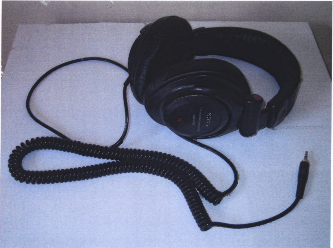
Figure 3.9 Pictured here are the stereo headphones (Model: Sony MDR-V600) used for auditory feedback of the participants' speech, in real time, while speaking.
