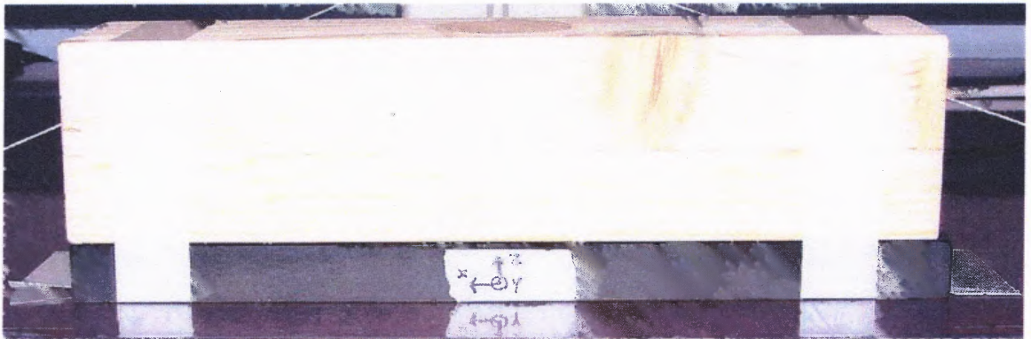
Figure 3.16 Force plate runway with isolator attached.
