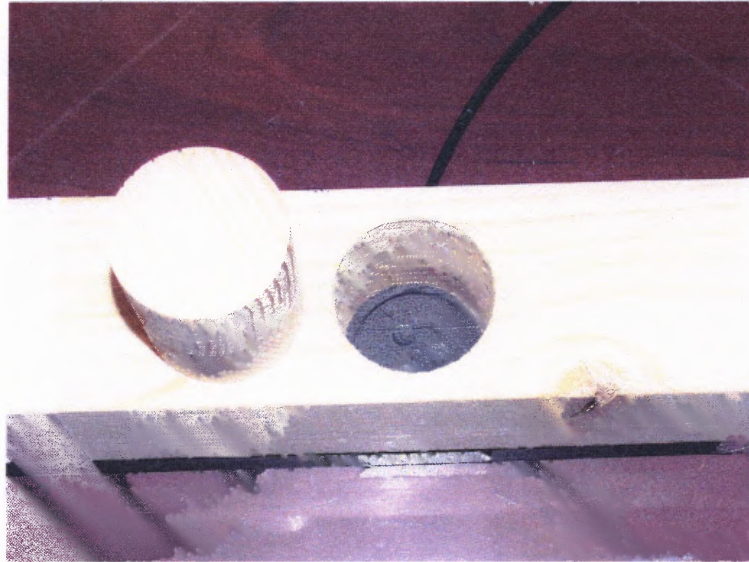
Figure 3.5 Wooden isolator mounted on force plate runway with plug removed.
