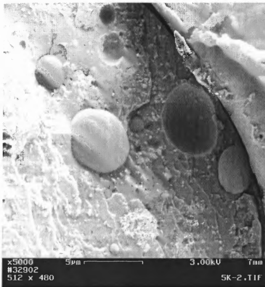
Figure 5.31c SEM of the fracture surface of unreacted 5PP/3UP containing MgO (15mins processing, 220°C, x5000).
