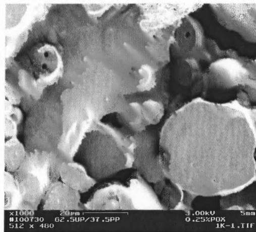
Figure 5.23b SEM of reacted 3PP/5UP (0.25phr POX, 15mins processing).
