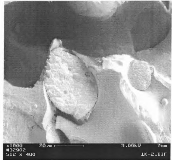
Figure 5.31b SEM of the fracture surface of unreacted 5PP/3UP containing MgO (15mins processing, 220°C, x1000).
