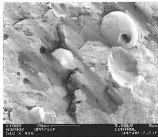
Figure 5.25a SEM of the fracture surface unreacted 3PP/5UP (blank, 15 mins processing).
