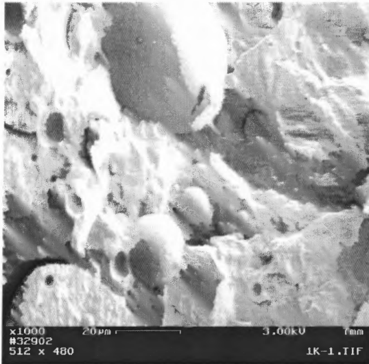
Figure 5.31a SEM of the fracture surface of unreacted 5PP/3UP containing MgO (15mins processing, 220°C, x1000).
