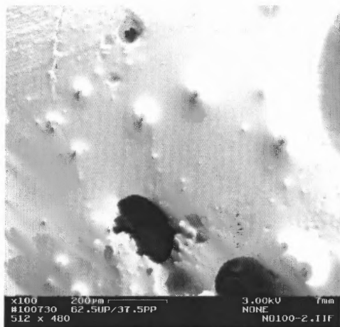
Figure 5.23a SEM of unreacted 3PP/5UP (blank, 15mins processing).
