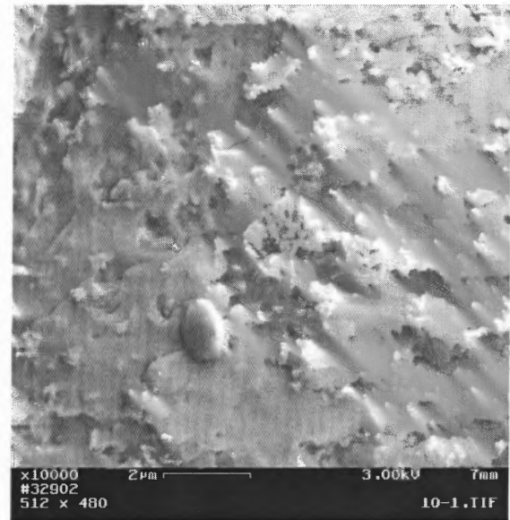
Figure 5.31d SEM of the fracture surface of unreacted 5PP/3UP containing MgO (15mins processing, 220°C, x10000).
