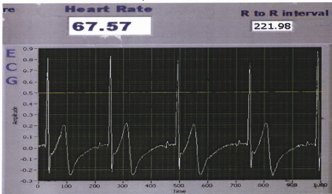
Figure 2.12 Front panel of the ECG graph with a user moveable threshold line.
