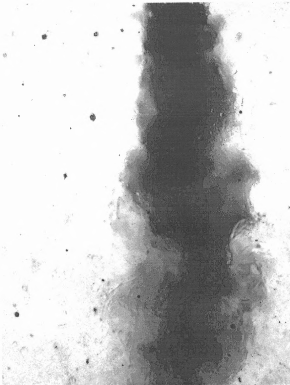
Figure E.9 Injection of solution into the view cell, P = 100 Bar, T = 35 C, V_{\text{sol}} = 0.4 ml/min, v = 1.18 m/s, D_{\text{nozzle}} = 254 \mu\text{m} , V_{\text{CO}_2} = 60 , \text{CO}_2 is injected with pulsations using 20 rpm pump.
