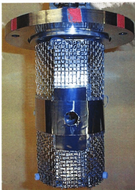
Figure 2.14 The Faraday cage mounted to the top flange of the sample chamber encloses the sample block.
