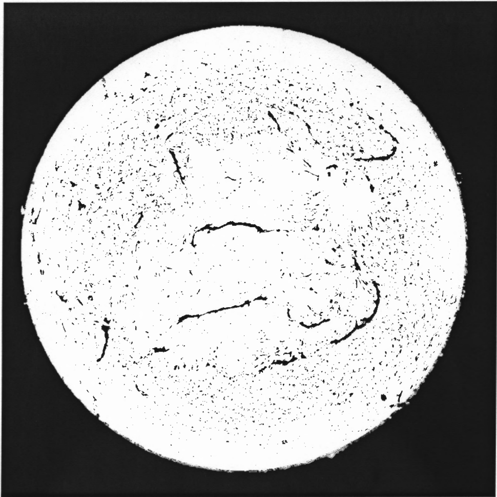
Figure A.25 Solar disk, advanced local thresholding, with asymmetrical cutoff values c_{\text{inf}}=50 , c_{\text{sup}}=155 , window size w=20 and modifying factor m=0.95 .
