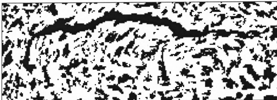
Figure A.20 Filament, advanced local thresholding c_{\text{inf}}=50 , c_{\text{sup}}=205 , window size w=20 .
