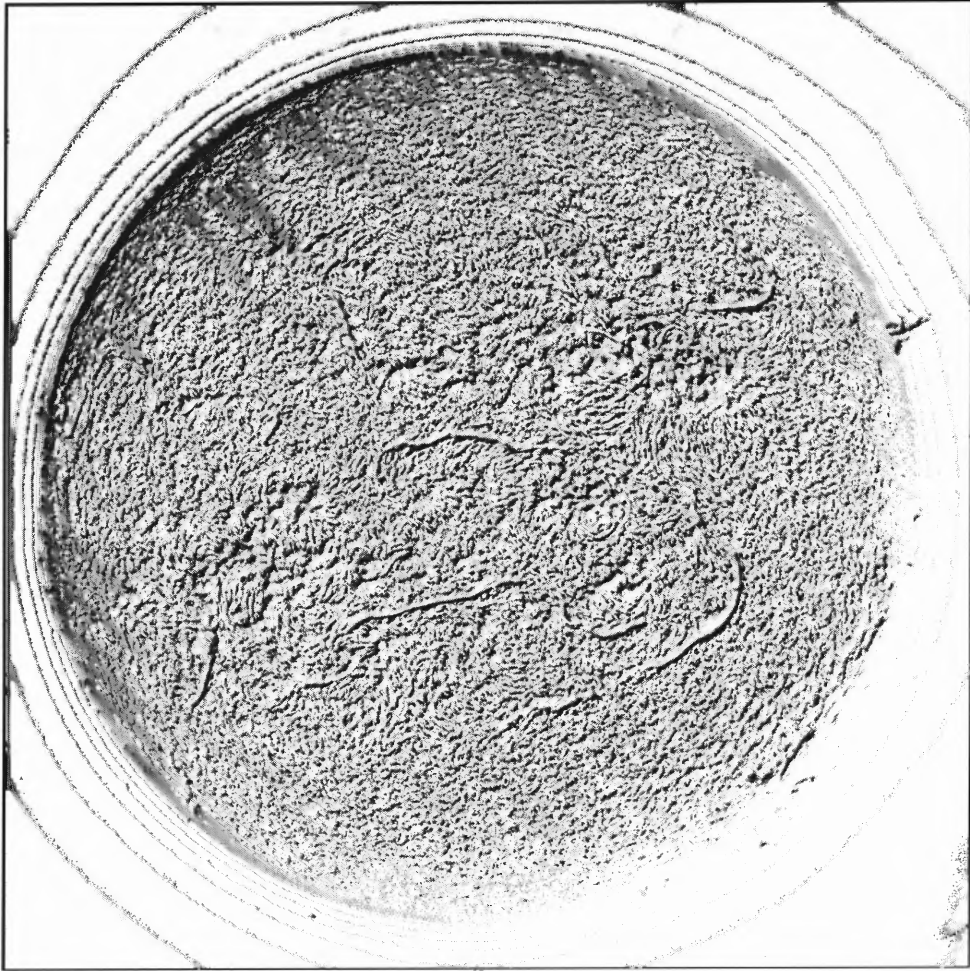
Figure A.7 Solar disk, smooth local histogram equalization, window size w=5 pixels.
