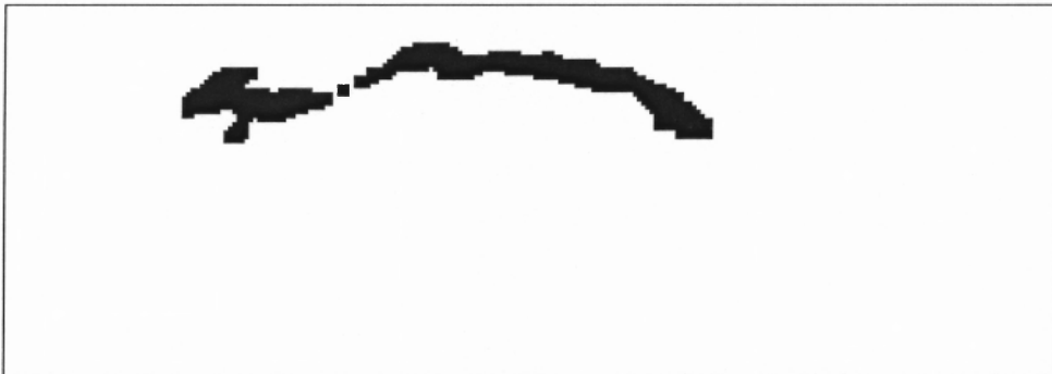
Figure A.48 Filament, preprocessed image, superposition of eight recursive directional closing operations, 3 \times 3 “cleaning” closing.
