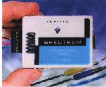
Figure 2.2 Spectrum SP-1700 thermocouple temperature data logger.
