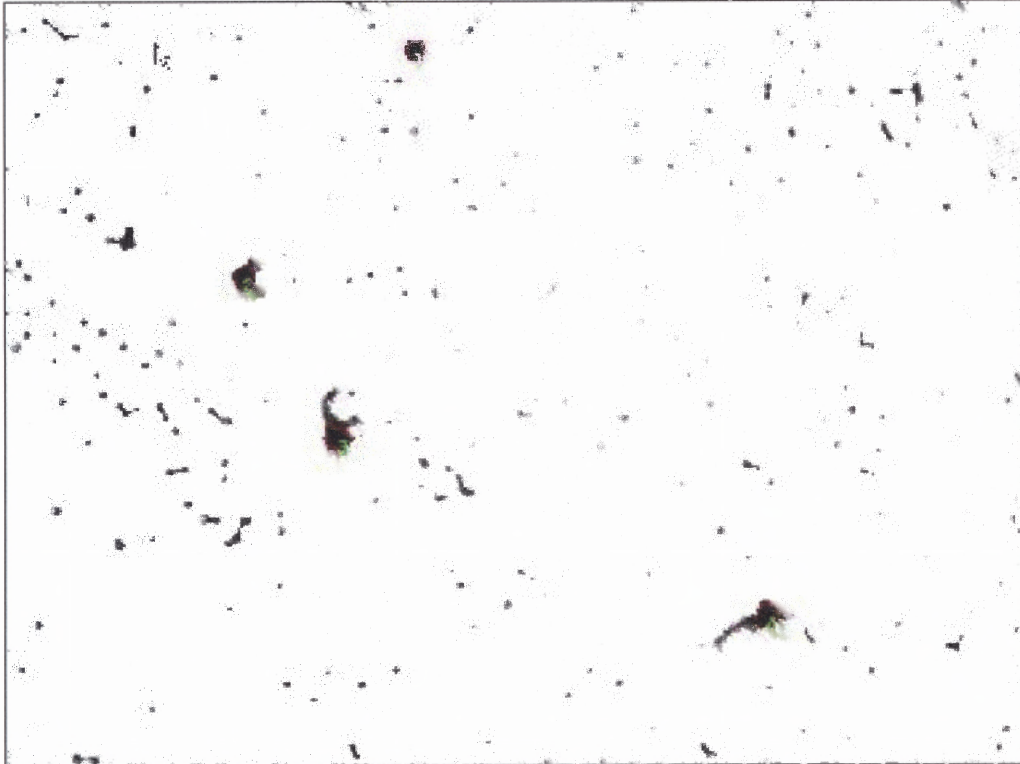
Figure 5.8 Image used in Step 4 for counting micropipes with Image-Pro.
