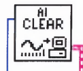
Figure A.3 AI Clear.vi in LabVIEW. AI Clear.vi empties the buffer at the end of the program.
