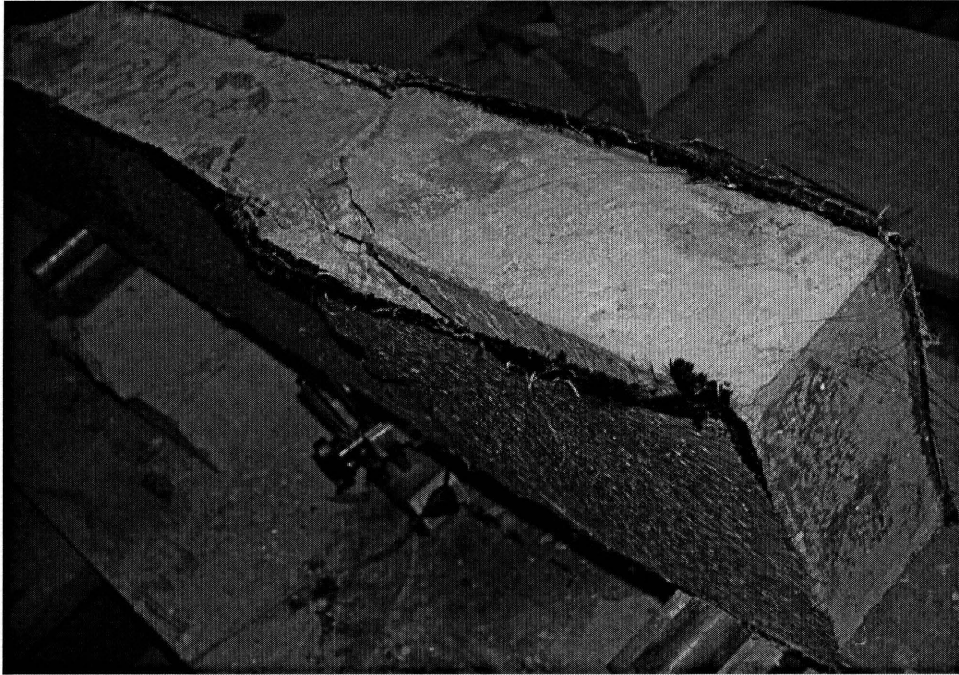
(b) Top View of the Beam at Failure
