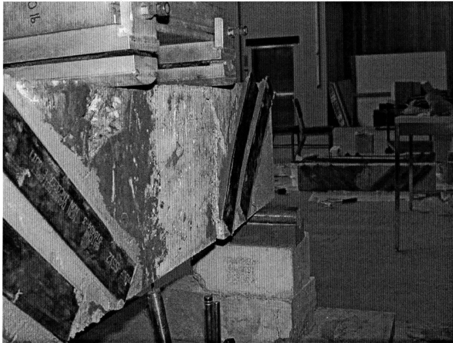
Figure 6.3 Failure of Beam Z22-SCR45.
