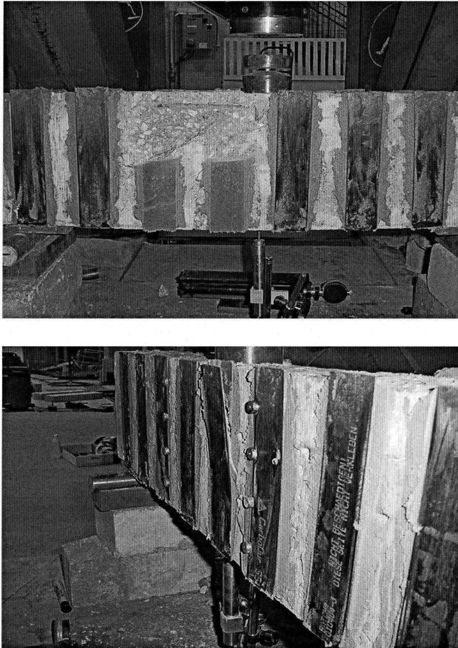
Figure 4.10 Failure of Beam Z11-S90.
