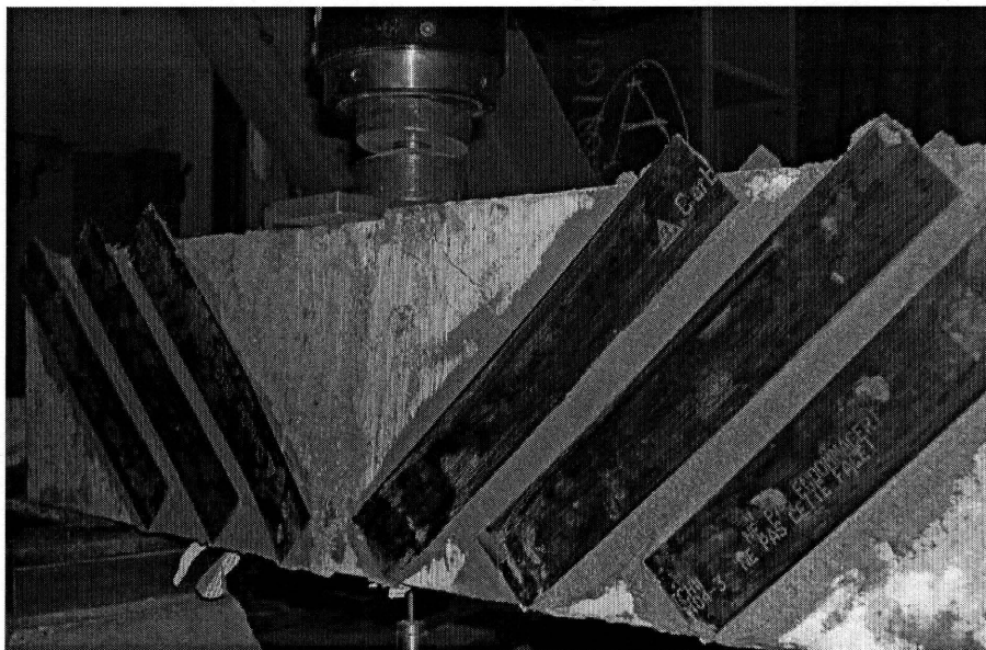
Figure 6.2 Failure of Beam Z11-SCR45.
