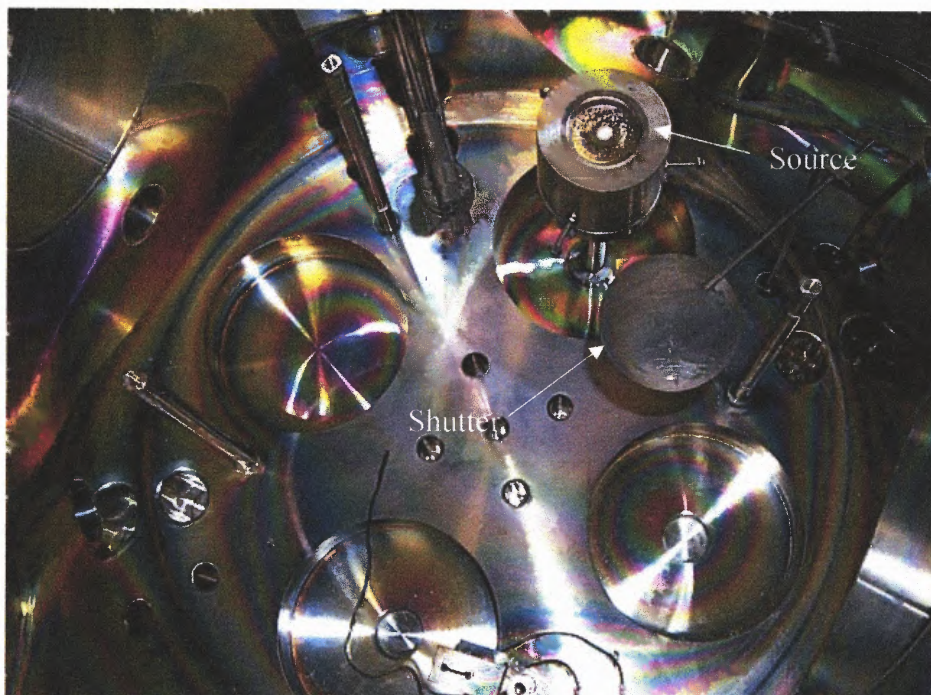
Figure 3.3 Inner view of the chamber showing the Torus 2 magnetron source.
