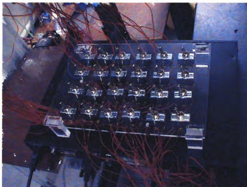
Figure 3.25 24-switch device and OMB-MultiScan 1200 system.
