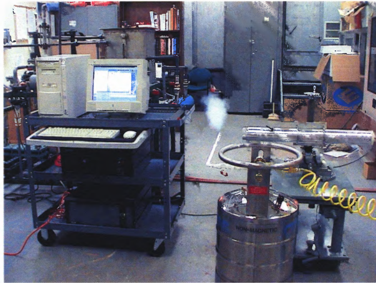
Figure 3.13 Calibration of pressure-controlled spray system.
