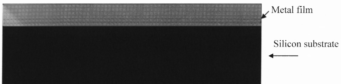
Figure B.1 Sputtered metal film on top of a silicon wafer.
