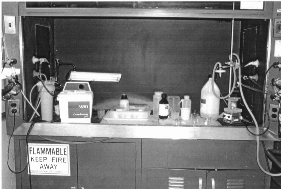
**Figure 6.5** Chemical station for etching.
