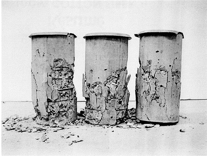
Figure B.7 Cylinder after Compression Test (Hoop S=1 in.)
