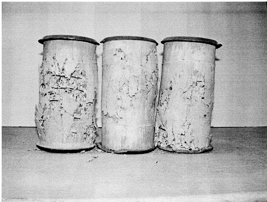
Figure B.8 Cylinder after Compression Test (Hoop + Steel Fiber)
