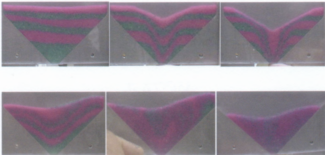
Figure 5.18 Snapshots of Hopper discharge without vibration (a)-(c), and with vertical vibration (d)-(f) showing mixing and mass flow characteristics
