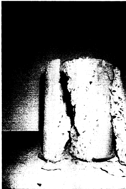
Figure 4.13 Mode of failure of high performance concrete.
