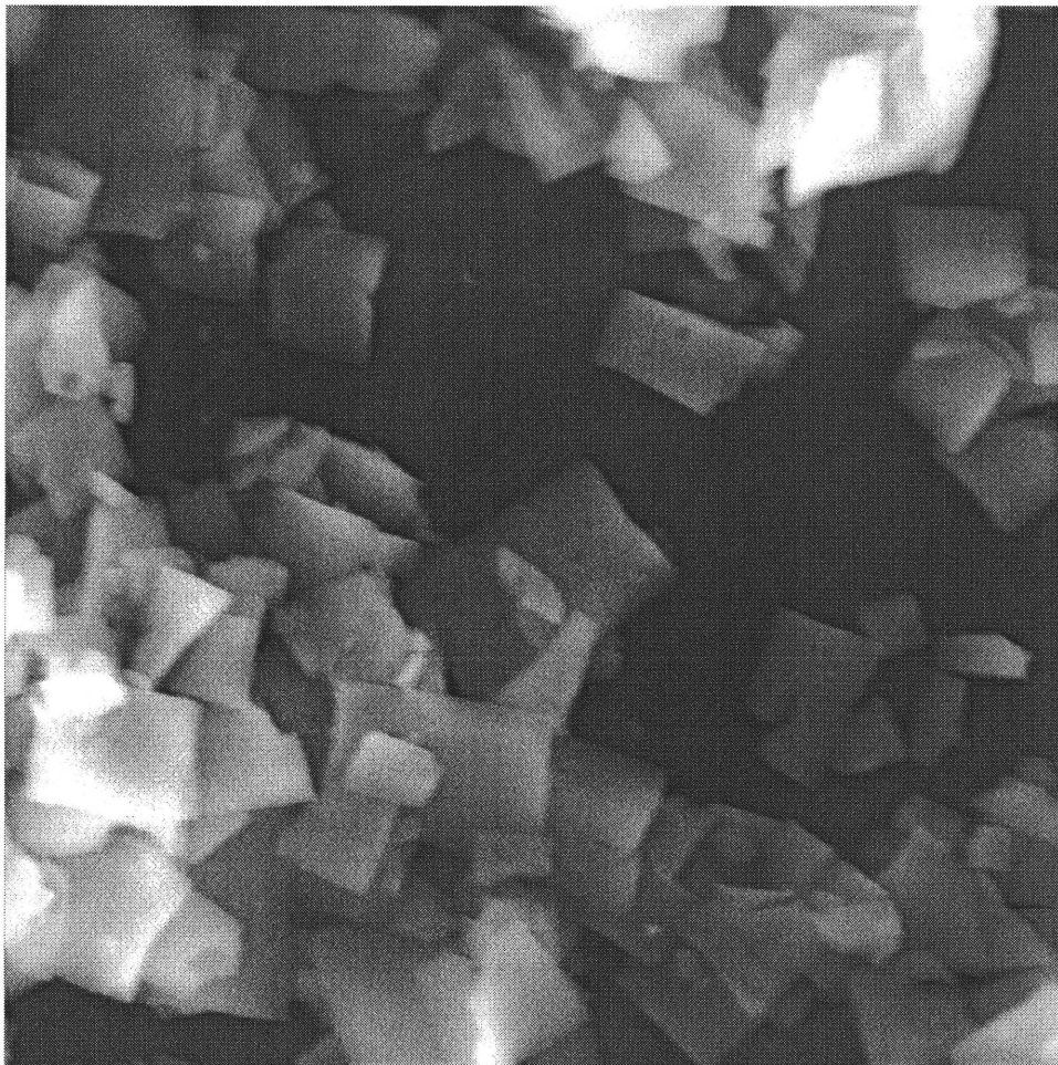
Figure A.21 Crystal shape for experimental design EDA6-Feed I t_f = 45 min, \alpha_w = 50 , C_{BOM} = 0.0045 kmol/m 3 , \eta = 1 , D = 0.076 m, C/T = 0.33 , N = 500 rpm: d_{43} = 6.05 \mu m, C.V. = 0.2567
