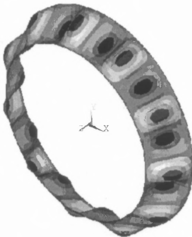
Figure 5.4(a) Deformed shape for L/R_1=0.5 , \alpha = 30^\circ , SS2 under outer pressure
