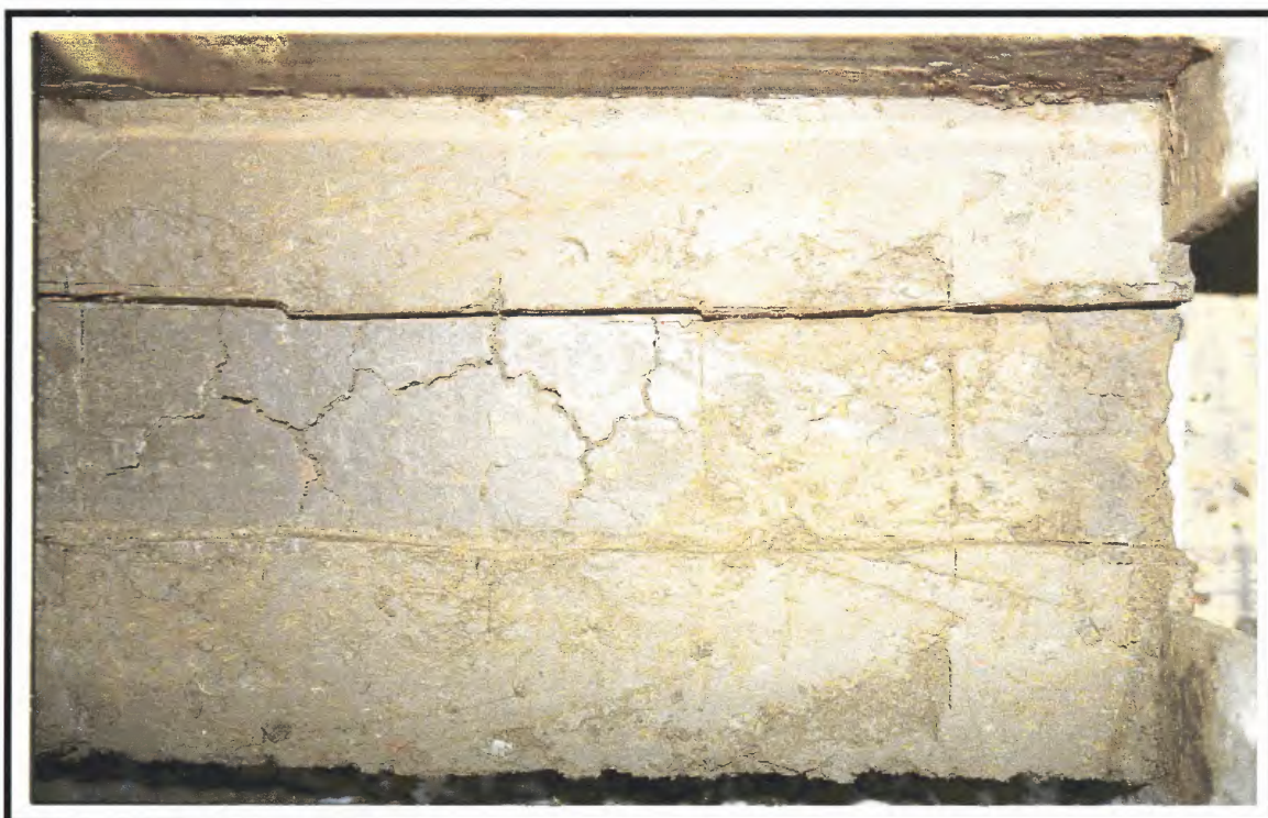
Photograph A-16. Note that the wetting also caused the vertical shrinkage cracks to seal at the fracture level.
