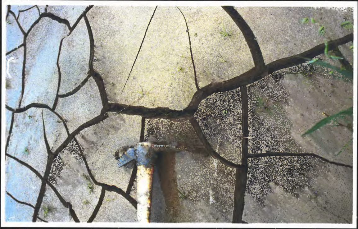
Photograph A-2. Shrinkage cracks in Potomac Formations clay, Rainwater Landfill, Lorton, VA. The end of the mattock is 15 in. long.
