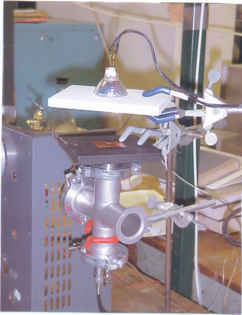
Figure B.4 View of Experimental Apparatus II. The distance of the light source from the filter is approximately 2.5 inches.
