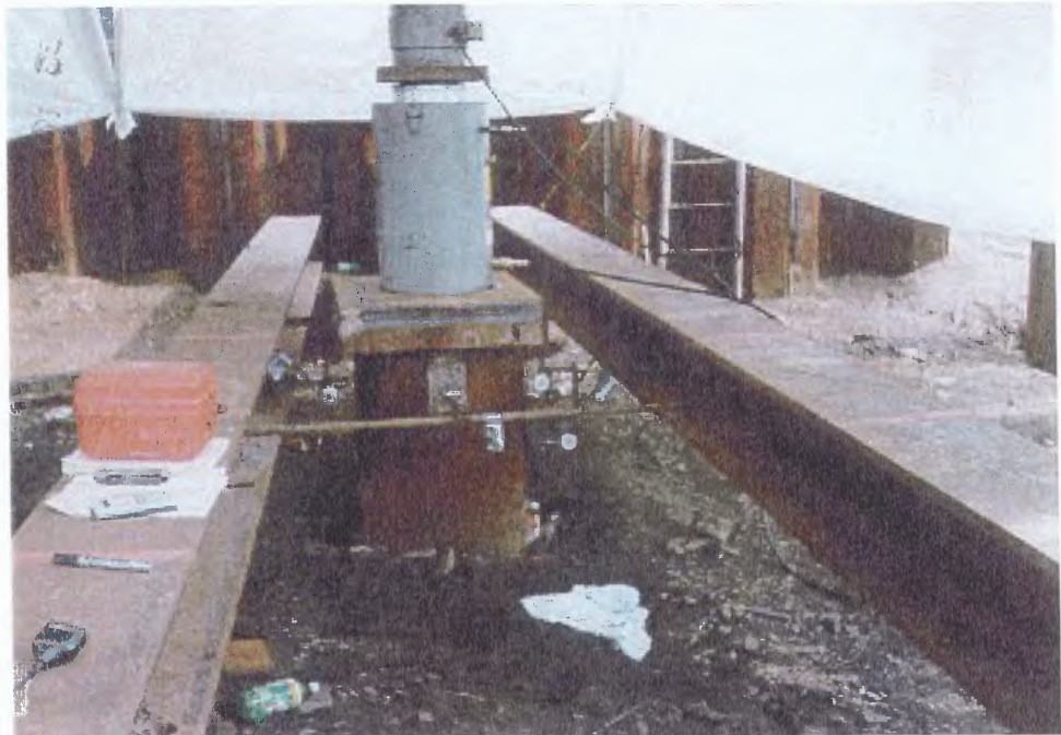
Figure 3.6 Static Load Test Setup
