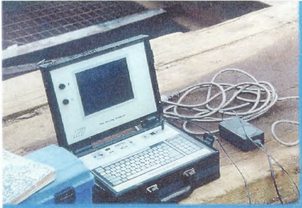
FIGURE 3.1 Pile Driving Analyzer Assembly
