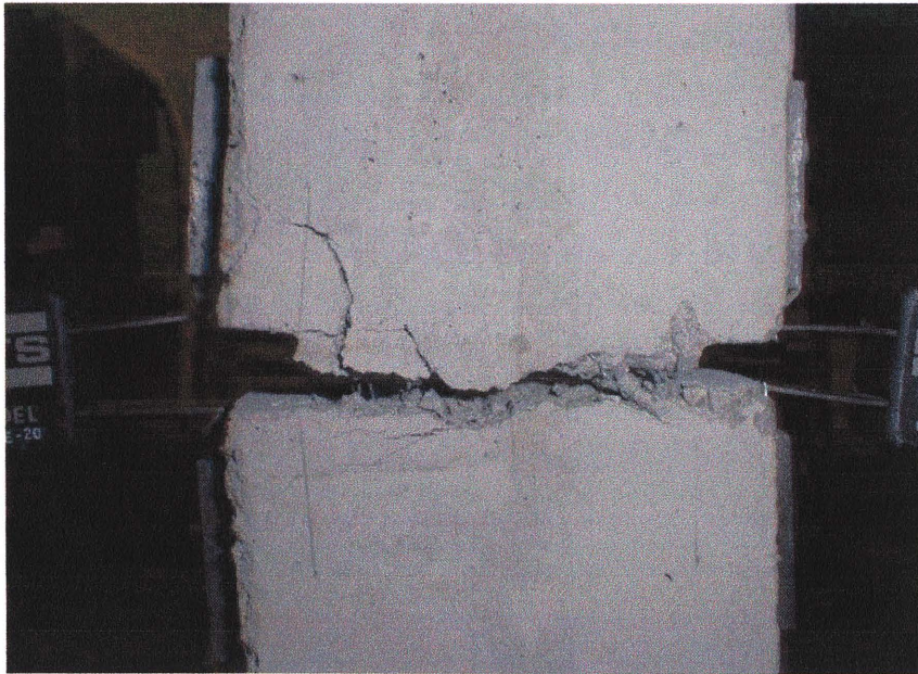
Figure 4.1(c) The Development of Multiple Cracks at Critical Section of the Specimen
