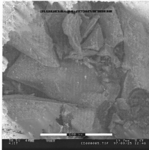
Figure 5.8 Morphology of Vitrified Soil from CD
