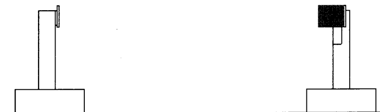
Figure C.2.1 Antenna Anechoic Test Chamber. The antenna on the left is the receiver calibrated antenna, the one on the right is the antenna under test.
