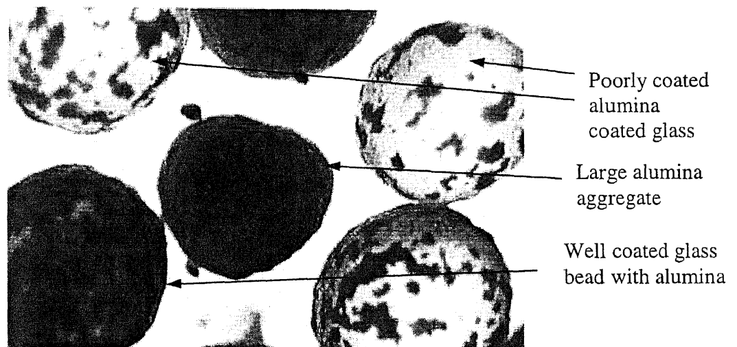
Figure 2.4 Optical microphotograph of DCSMM process for 2 hours: Alumina = 1g, Glass beads = 5g Observation: Some particles are well coated and some are poorly coated, and compaction of alumina is manifested by formation of large aggregates.
