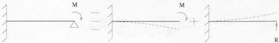
Figure 3.5 1D Cantilever beam model.
