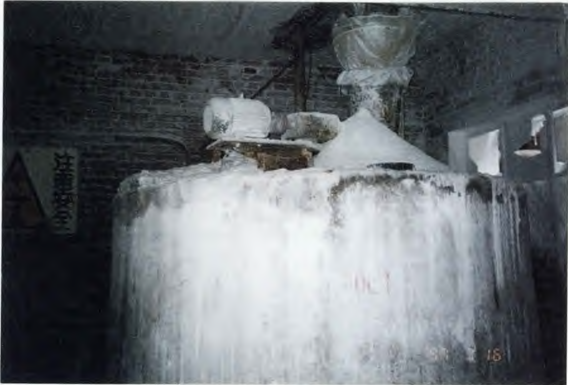
Photograph 3. Preparing the Pulp - Dispersion in Water
