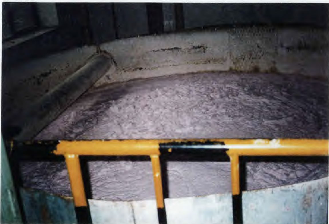
Photograph 4. Adding Additives such as Talc and Silicas
