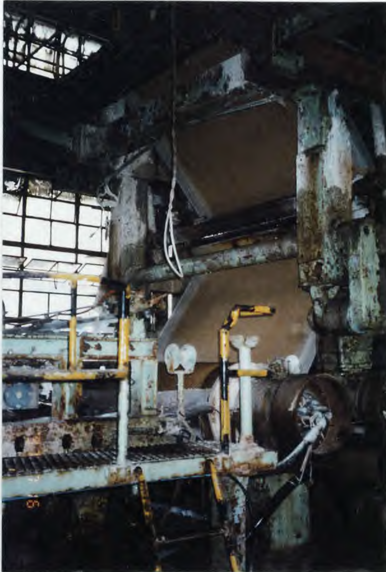
Photograph 12. The Wire-Mesh Conveyor Belt as it Moves and Transports the Slurry between the Rollers
