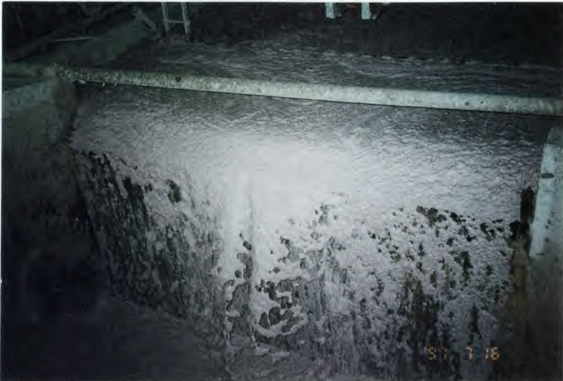
Photograph 6. Slurry before it is Transported to the Paper Machine
