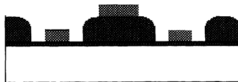
Figure 3.4f The polysilicon was patterned and RIE etched as shown. This polysilicon over the active area acts as a self-aligning mask during the formation of the source and drain.
