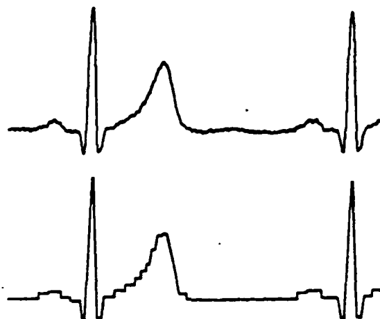
Fig. 1. ECG sampled at 500 samples per second (top) and resulting AZTEC representation (bottom) as reproduced by a digital plotter. The horizontal line at the upper left indicates 100 ms and the vertical line indicates one eighth of full scale, in this case 400 \mu V.
