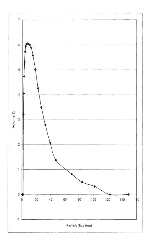
Figure 6.5: Particle Size after Sonication for 60 seconds
