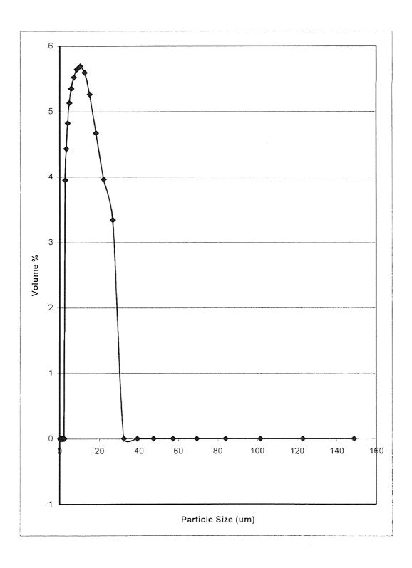
Figure 6.4: Particle Size after Sonication for 30 seconds
