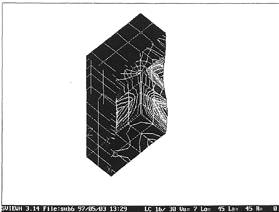
Figure G.16 Enclosure Mode Shape 16: f = 870.25 Hz
