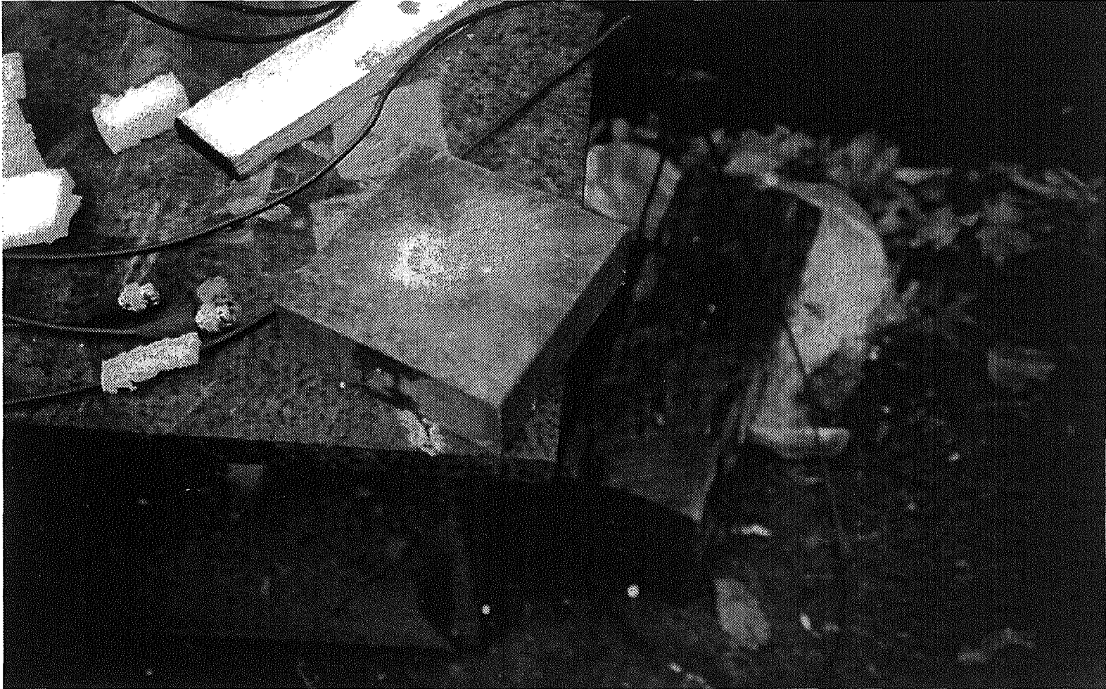
Figure 46 Witness Plate After Explosive Test
