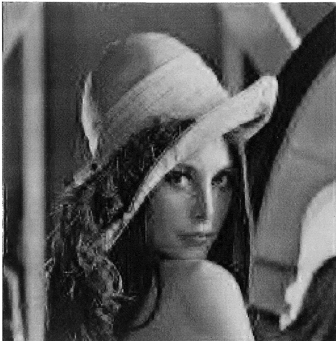
Figure 5.10 (b) Compressed “lena” Image by Vector Quantization with Codebook II at R = 0.40 bpp, SNR = 27.48 dB (Binomial PR-QMF Bank).
