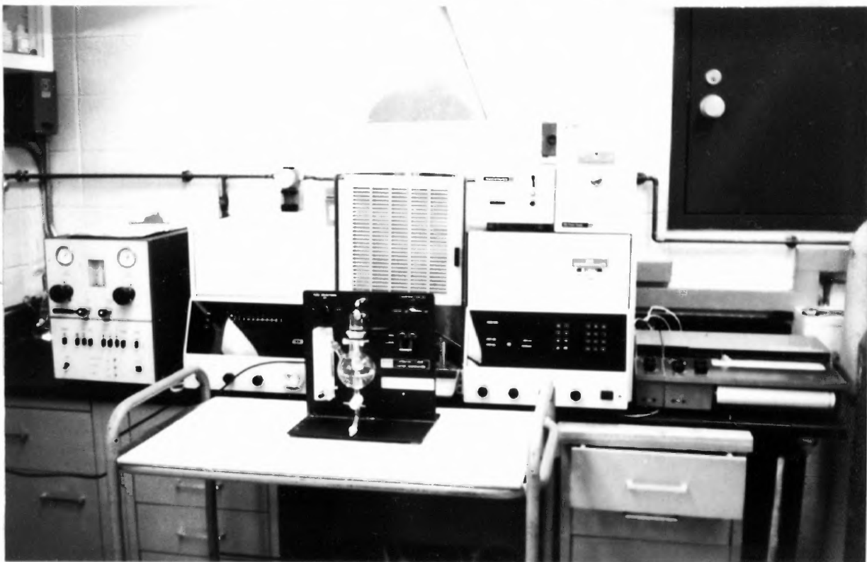
Figure 3b Picture of Perkin Elmer Model 603 Atomic Absorption Spectrophotometer with Cold Vapor Generator Setup for Arsenic Analysis via Hydride Generation
